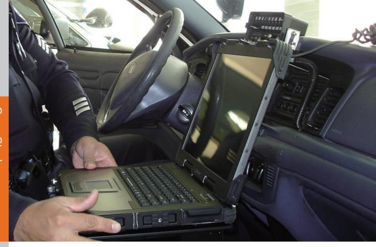
Getac docking station allows our officers the flexibility of removing the unit from the vehicle and working from a more comfortable or convenient location.
